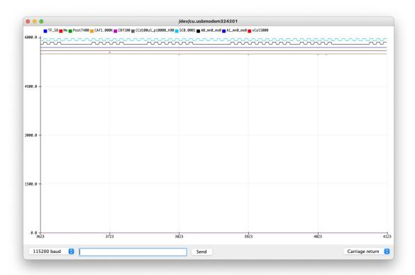
Notice the top line is what we expected, the second line with pulses only sometimes is due to it floating. You can either just connect the unused inputs to ground or ignore the traces.
