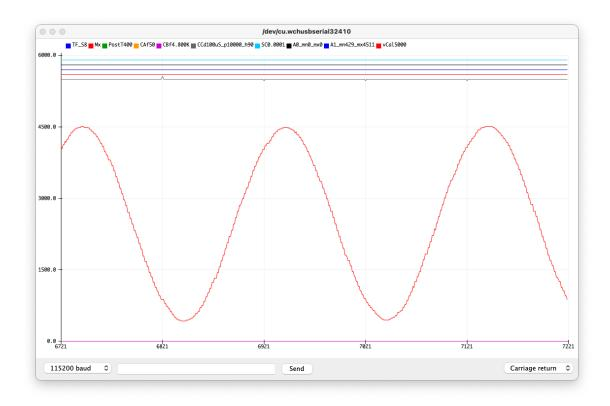
The frequency limits are significant. Going up to 1K already makes the ability to get any phase information difficult.
