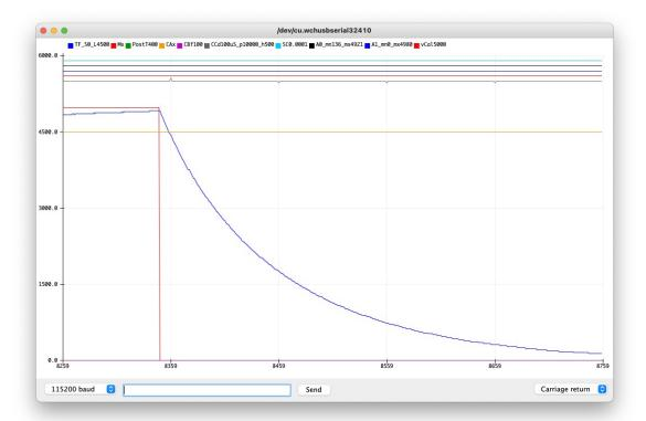
I now need to set the measure point to be at another voltage of the A0. I will just pick falling through the 0.5 volt level. So commands are MS0, MF, and ML500.
