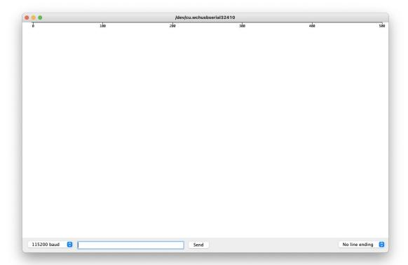
In the Arduino environment under Tools clock on the Serial Plotter option. It will open up another window. Notice that in the lower right corner it says "No line ending". Click on that and change it to "Carriage return". Change the baud rate to 115200 if it not already set to that. Now just click on the "Send" button.
