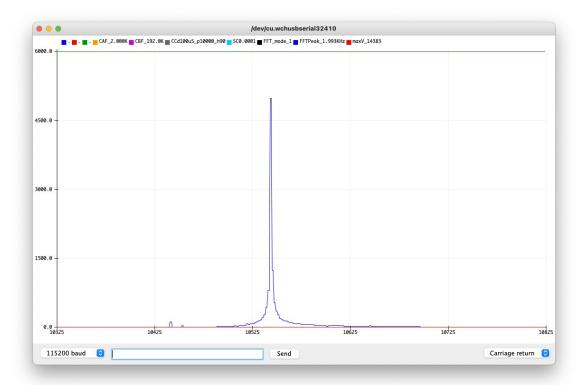
Notice the status line has changed significantly. It does tell us that we are in FFT mode 1 and that the peak is at 1.993KHz. The maxV is a bit less useful. But the plot does show one peak really close to the expected 2KHz.
