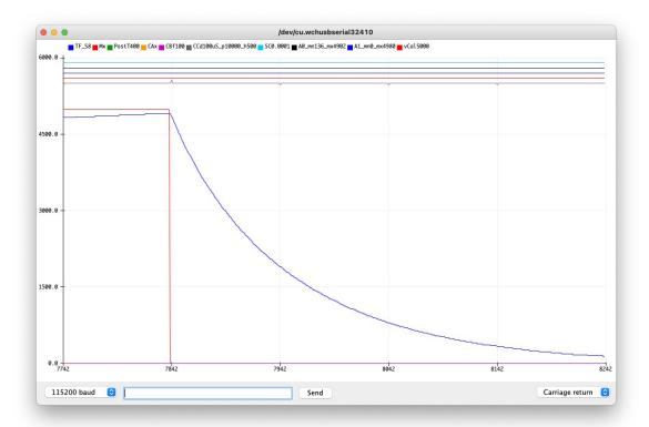
I would like to time the drop between 2 known voltages. So I want the trigger to be at a known point. I just picked 4.5 volts as something easy to see. So to fix the trigger we use TS0 to say watch channel 0. Then commands TF and TL4500 (or a single command TF4500) to say we want trigger falling at a level of 4.5V.
