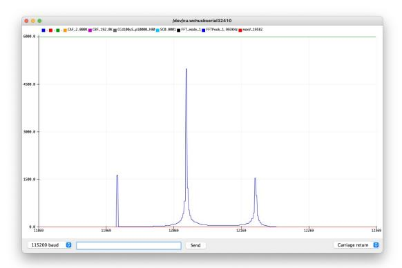
Even though we are feeding in the same frequency, it is a square wave, we now see other peaks. Use the CSF500 to drop the frequency down to 500Hz and re-plot it.
