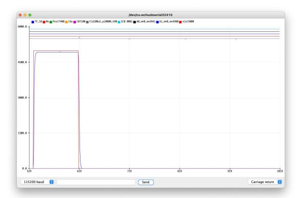
We now have a plot. There is a square pulse now. But there is also a not quite so square pulse that lags the original. This is caused by the A0 port not being connected to anything and the voltage on it just drifts around. Add a jumper from A0 to ground. Redraw the plot by clicking Send again.
