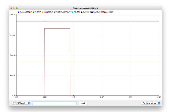
The commands for the measurement modes are nearly identical to the trigger modes. Note that the status line shows  $M_X$  to indicate that it is off. We want to watch for falling signal on A1, so we use the MF command to indicate falling and MS1 to use the voltage on channel 1. Note that the voltage level for the measurement point is set to 1000 or 1.000V. Hit another return to refresh the plot.
