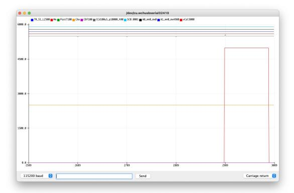
Notice there are 5 horizontal lines at the top of the plot. The top 4 are the digital inputs. The 5<sup>th</sup> one tells us where the trigger is. Notice there is a small upward spike where the trigger occurred.
